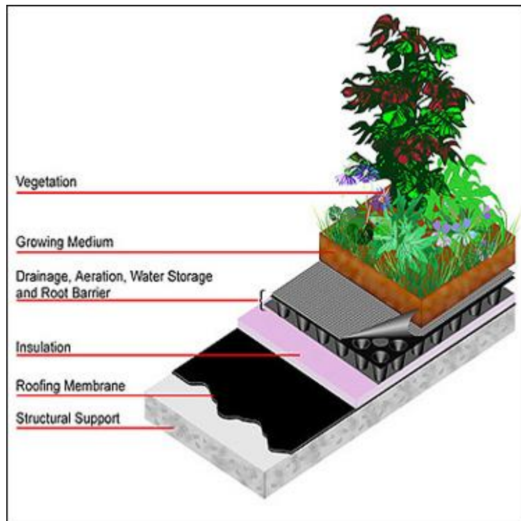
Figure 6 Green roof composition 11
