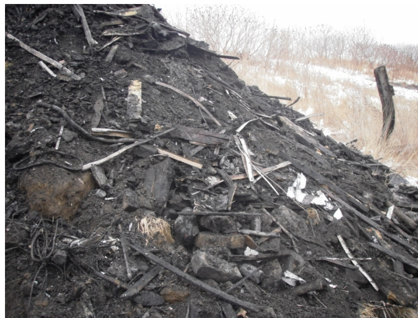
Wood and concrete debris mixed with soil and cinders.
