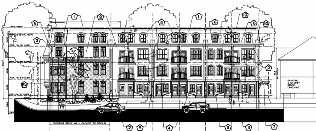
BLOCK B & C - NORTH ELEVATION FACING SYLVAN AVENUE SCALE: 1 : 150
