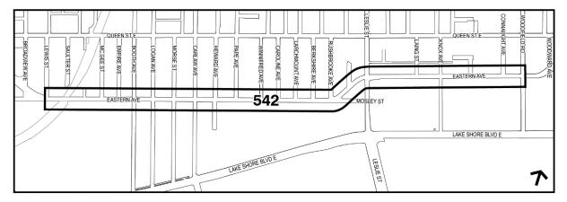
The planned right-of-way width for Eastern Avenue is 23.0 metres. The entire widening required to achieve this right-of-way width will be acquired from lands on the south side of Eastern Avenue.
