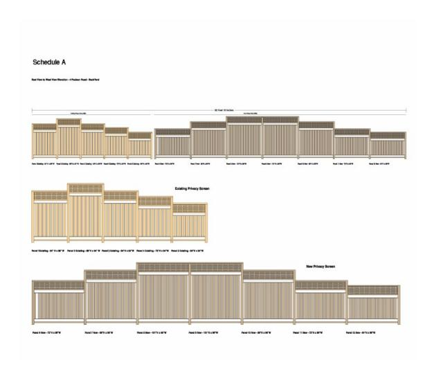
**Attachment 2:** Fence Details showing existing 5 panels and 7 new panels
