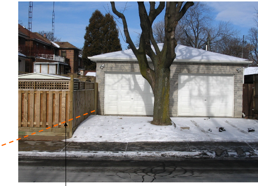
Fence required to be cut back at 45° angle to avoid sightline obstruction if tree is removed
