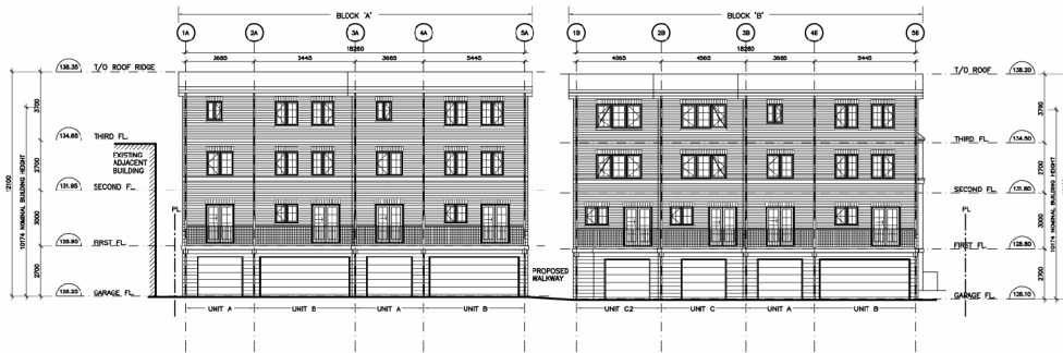
BLOCK A BACK ELEVATIONS
