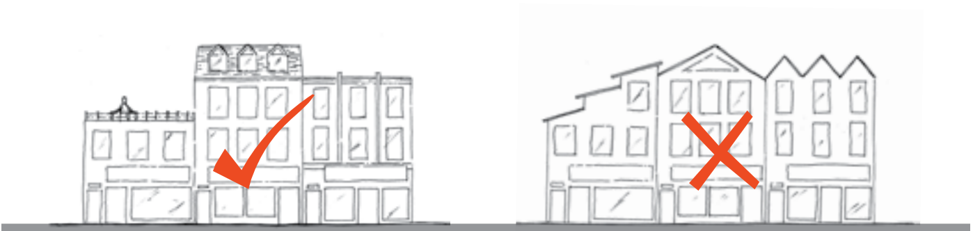
New buildings must present horizontal roof lines and/or roofs that slope towards Queen Street West.
