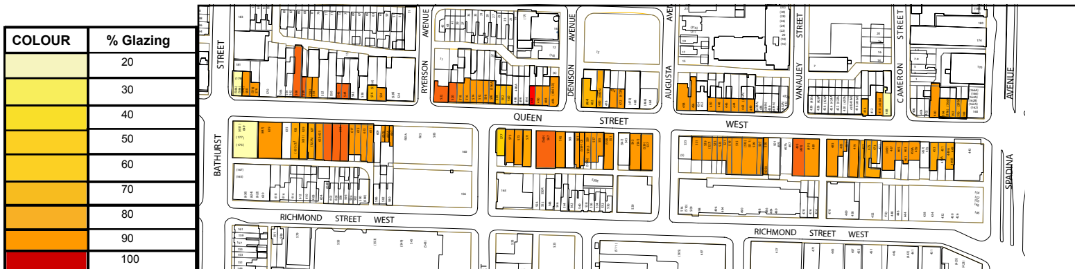
Ground Level Glazing in Contributing Buildings
