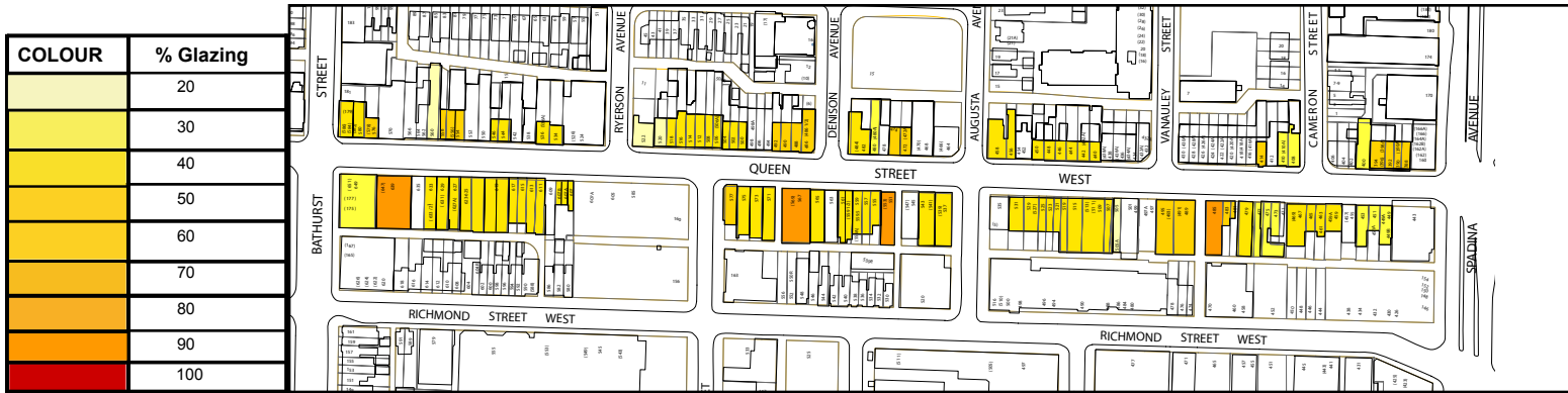
Upper Storey Glazing in Contributing Buildings
