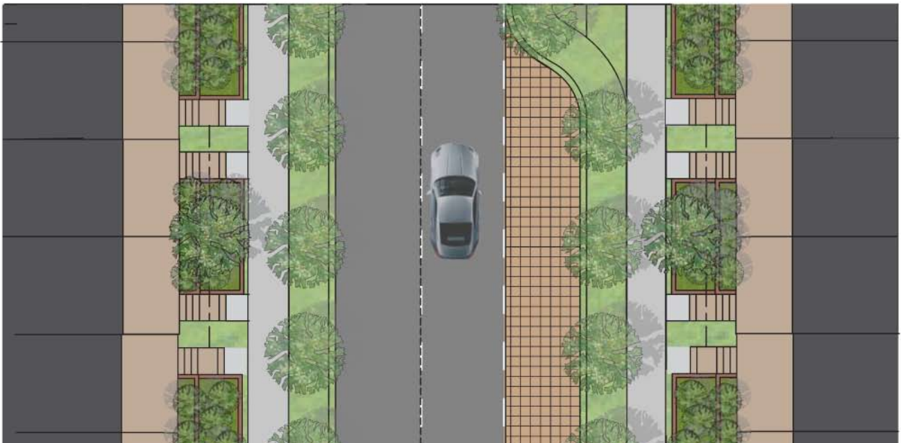
The Intermediate East-West Street 'C' has a right-of-way width of 18.5 metres and an asphalt width of 8.5 metres.
