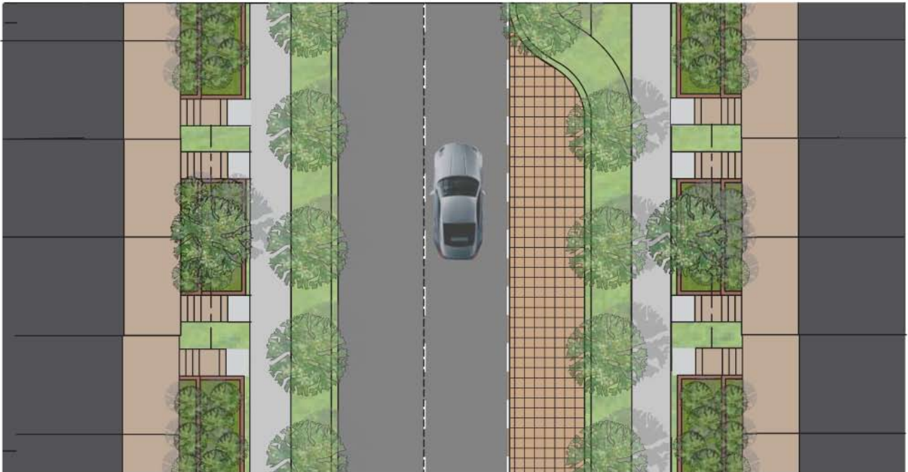
Intermediate North-South Street 'B' has a right-of-way width of 18.5 metres and an asphalt width of 8.5 metres.
