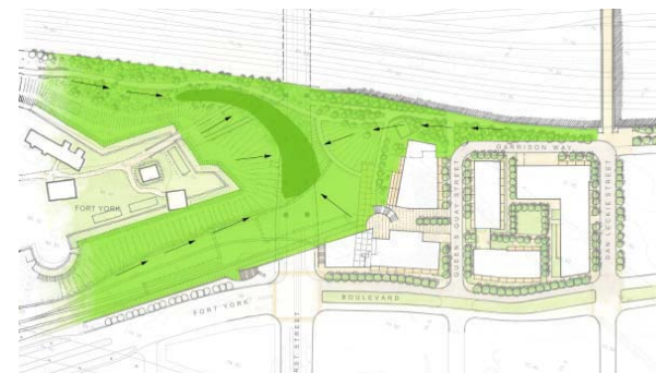
Stormwater Catchment Area
