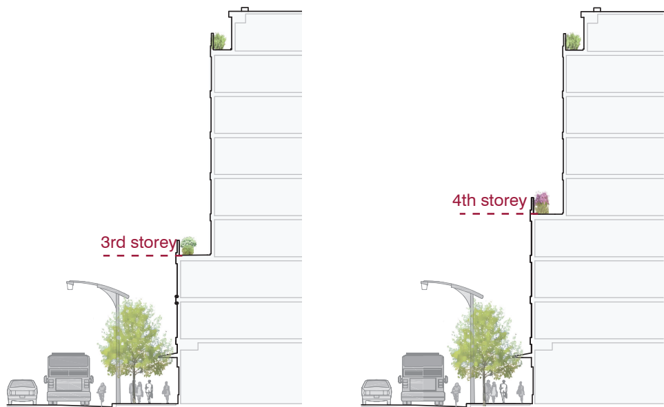
Range of alternative Pedestrian Perception step-back locations applied to a 9-storey building.
