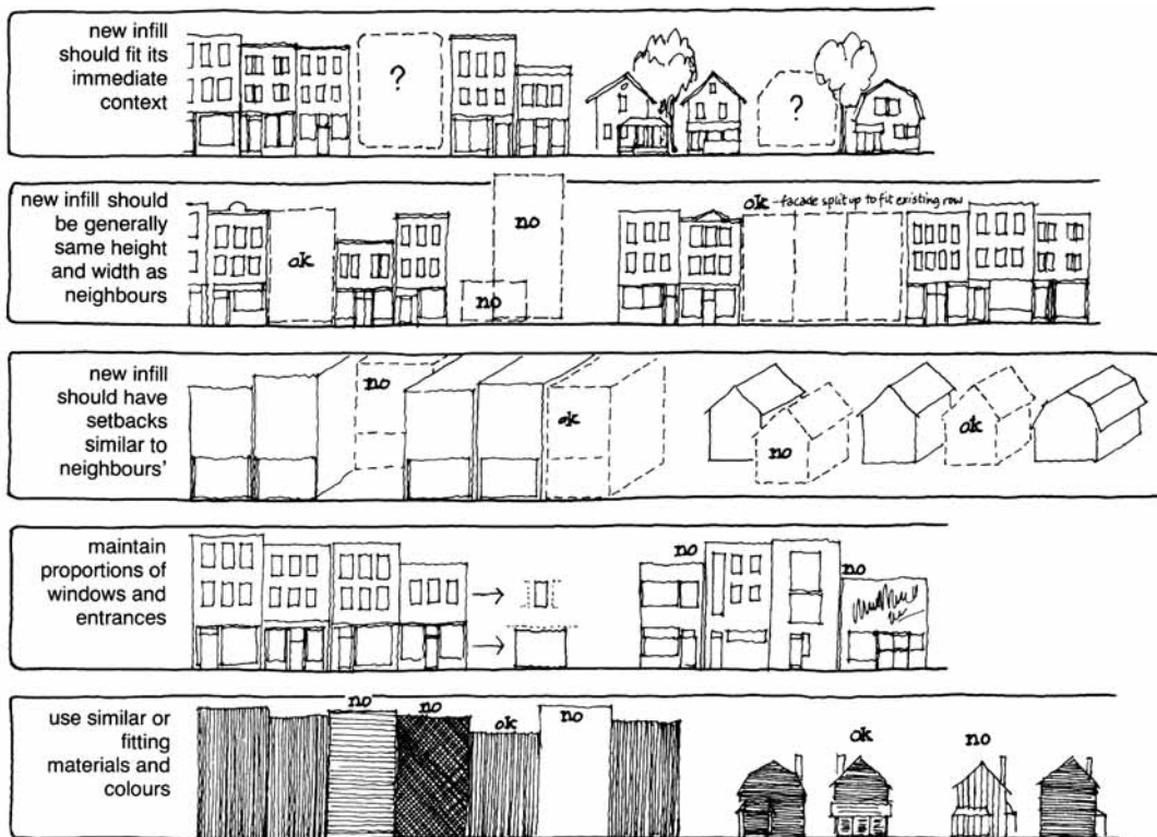
This is a good example of the use of simple graphic to demonstrate acceptable and unacceptable infill design. (Graphic: Ministry of Culture)
