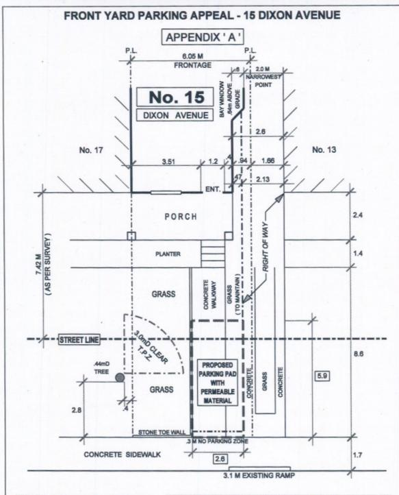
NOTE: PERMIT PARKING ON SAME SIDE NO LOSS OF PERMIT PARKING SPACE DUE TO USE OF EXISTING RAMP
