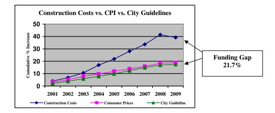
period increased by 18.8%. The chart below indicates the increased gap between the costs of construction, CPI, and the City's guidelines between 2001 and 2009.
