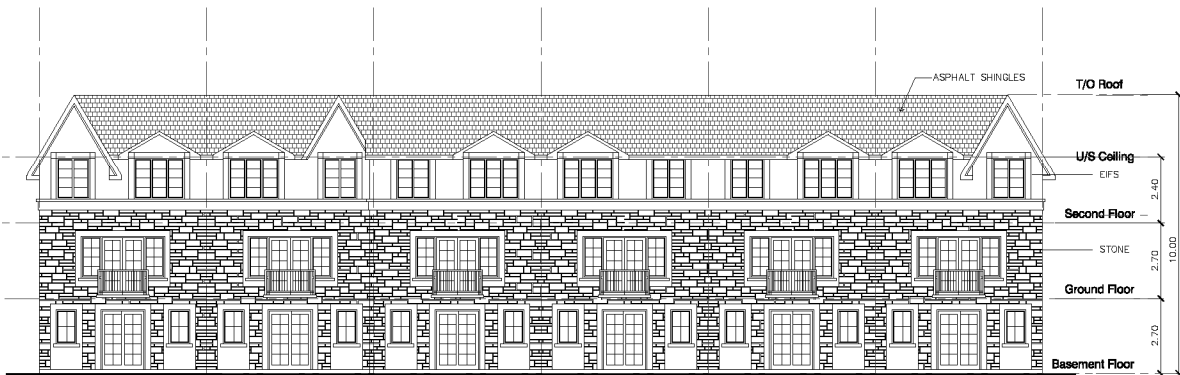
Rear Elevation 6-Unit Cluster
