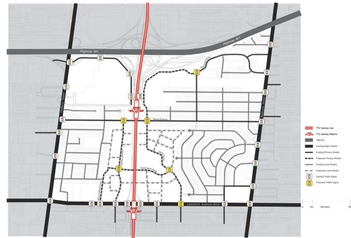
Figure 36: Possible New Signalized Intersections
