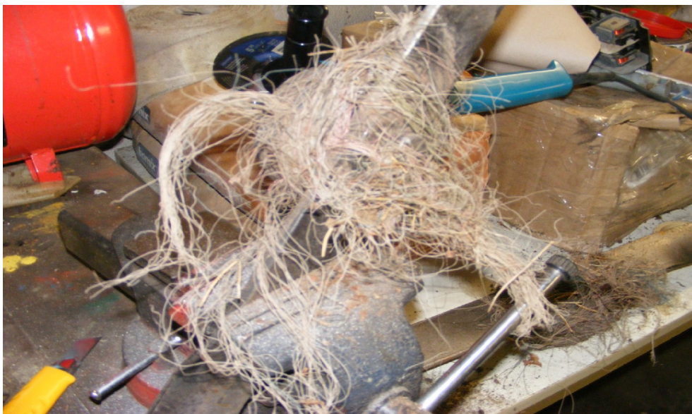
Damage to turf mowing equipment from abandoned kite line left on ground
