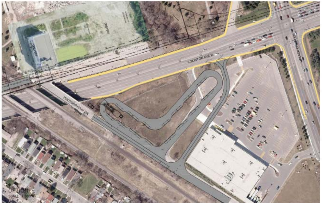
Figure 2-9: Bus Terminal Design Concept 2a – South Side, Single-Level Terminal
