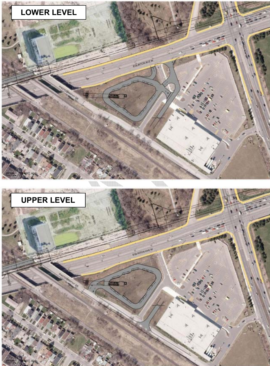
Figure 2-10: Bus Terminal Design Concept 2b – South Side, Two-Level Terminal
