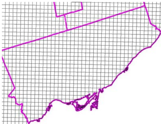
An example of grid cells in a Weather Research Forecast (WRF) model of 1 km x 1 km resolution used in evaluation of Toronto's future climate and weather.
