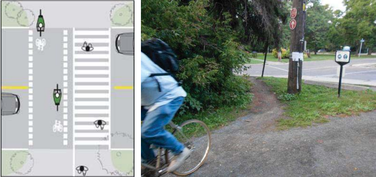
Left: Separated zones design is a best practice solution for crossings
