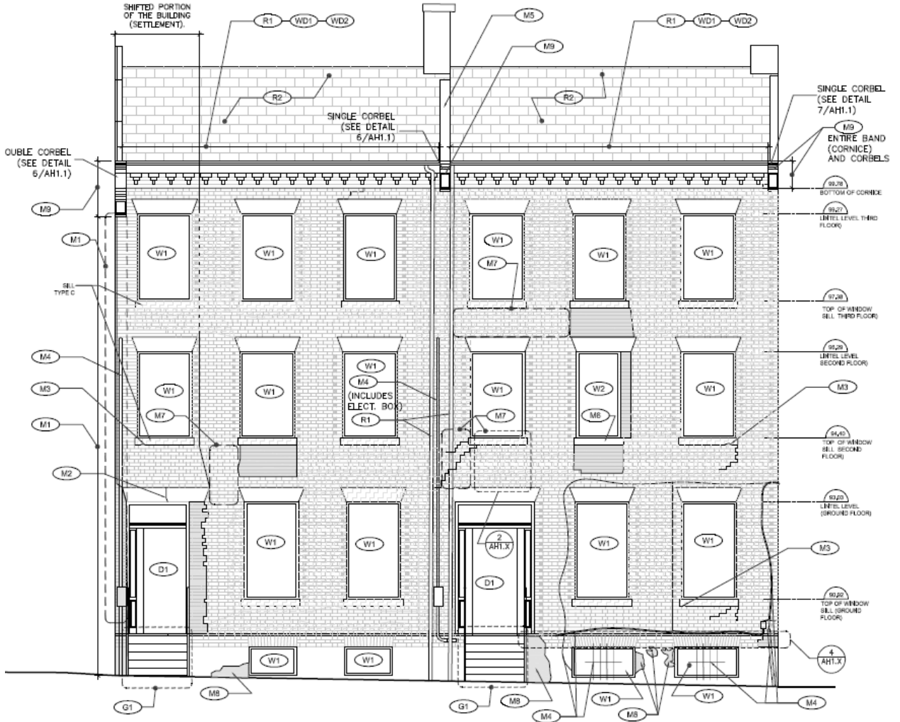
Assessment of the existing condition of the south elevation prepared by Goldsmith Borgal and Company Ltd. Architects. Areas of deterioration are identified.
