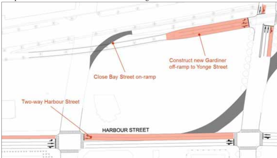
Figure 39 - Removal of the Bay Street on-ramp, new off-ramp to Yonge Street, and two-way Harbour Street
