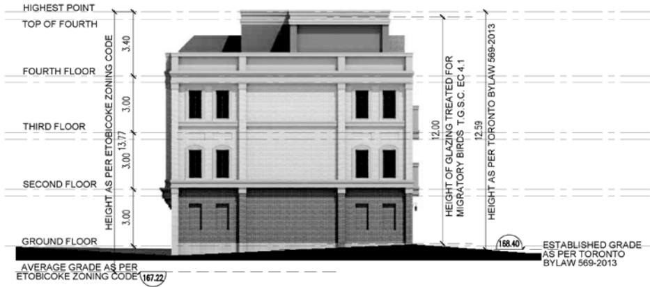
02 BLOCK 8 – EAST ELEVATION (SIDE) A302 STACKED TOWNHOUSE
