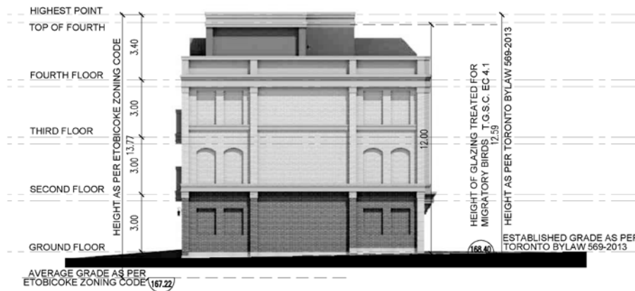
04 BLOCK 8 – WEST ELEVATION (SIDE) A302 STACKED TOWNHOUSE
