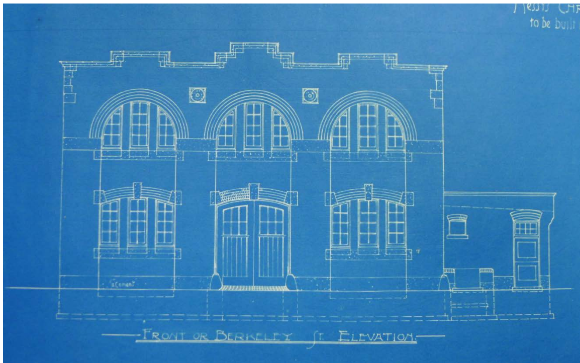
11. Sproatt & Rolph, "Front or Berkeley Street Elevation," (detail) 1905 : showing the main façade with the double storey arcade, the tri-partite windows of the upper story and in the distance the single storey elevation of the horse hospital (demolished). Note the double doors and ramp with protective bollards at either side of the carriage entrance. ( City of Toronto Archives )
