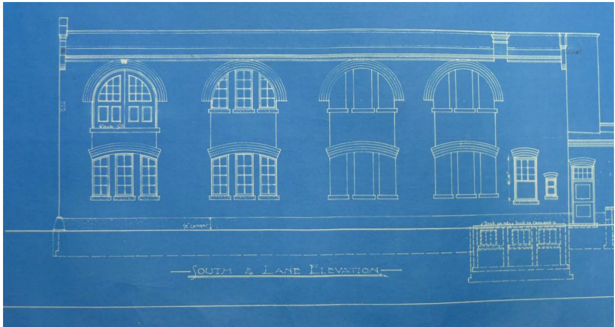
14. Sproatt & Rolph, "South & Lane Elevation" (detail) 1905: showing the south façade of the carriage building with the double storey arcade, and tri-partite 'thermal' windows. Note the double doors at the upper level for delivery of goods. ( City of Toronto Archives )
