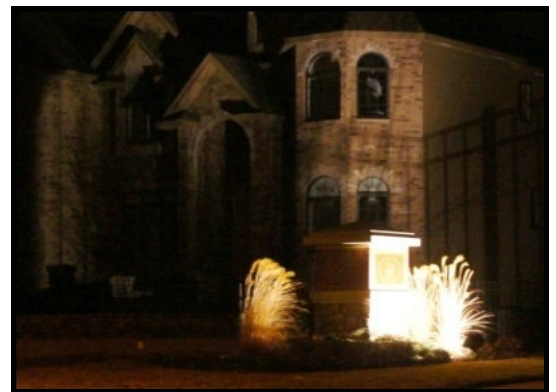
Light Overspill from Uplighting of Sign
