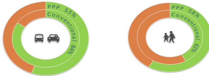
Figure 7 - Signal Time Allocation for Vehicles and Pedestrians at Pedestrian Priority Phase compared to a Conventional Signal
