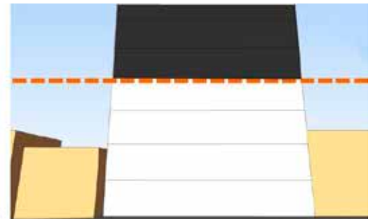
Loss of sky view due to increased height
