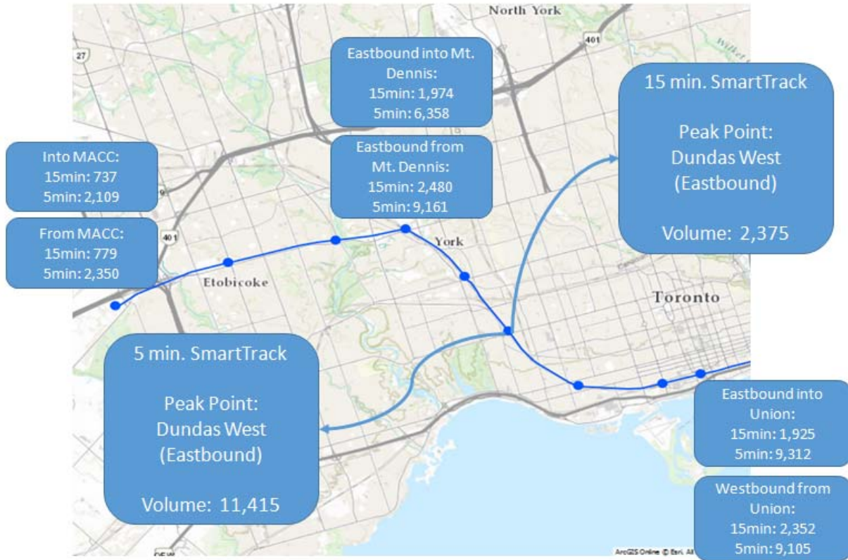
Figure II.1: 2031 AM-Peak-Hour, Peak Direction Volume: West Portion (assumes Low population/Medium employment with SmartTrack influence land use and TTC fare on SmartTrack)
