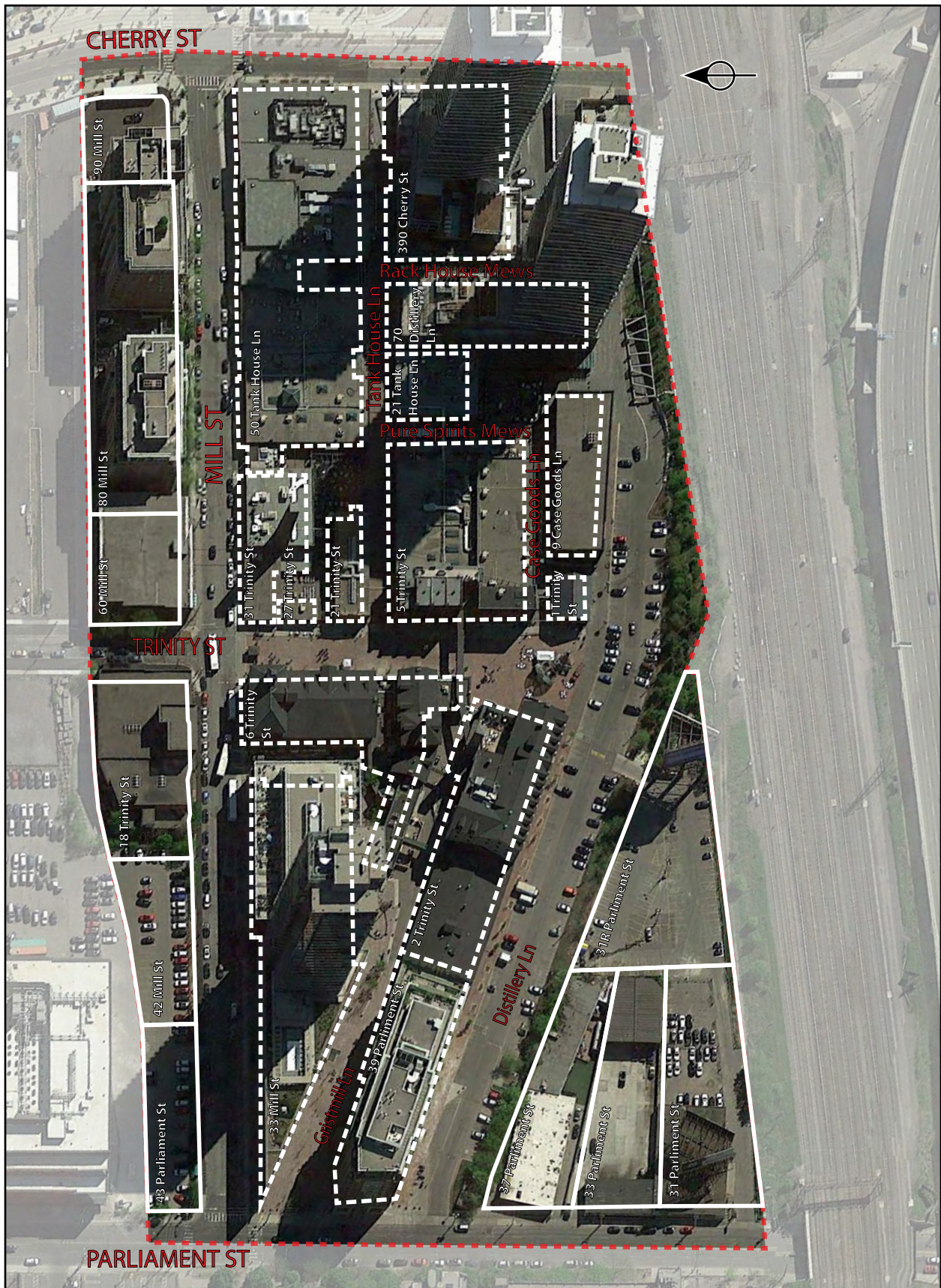
MAP. 13 PROPERTY PARCELS AND INDIVIDUAL STRUCTURES USING THE THA IDENTIFICATION SYSTEM. SOLID LINES INDICATE PROPERTY PARCELS SURVEYED, AND DASHED LINES IDENTIFY INDIVIDUAL STRUCTURES (GOOGLE/THA 2016).
