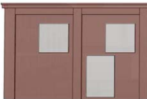
Distance between windows and brick pilasters: 200mm
