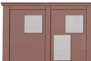
Distance between windows and brick pilasters: 200mm
