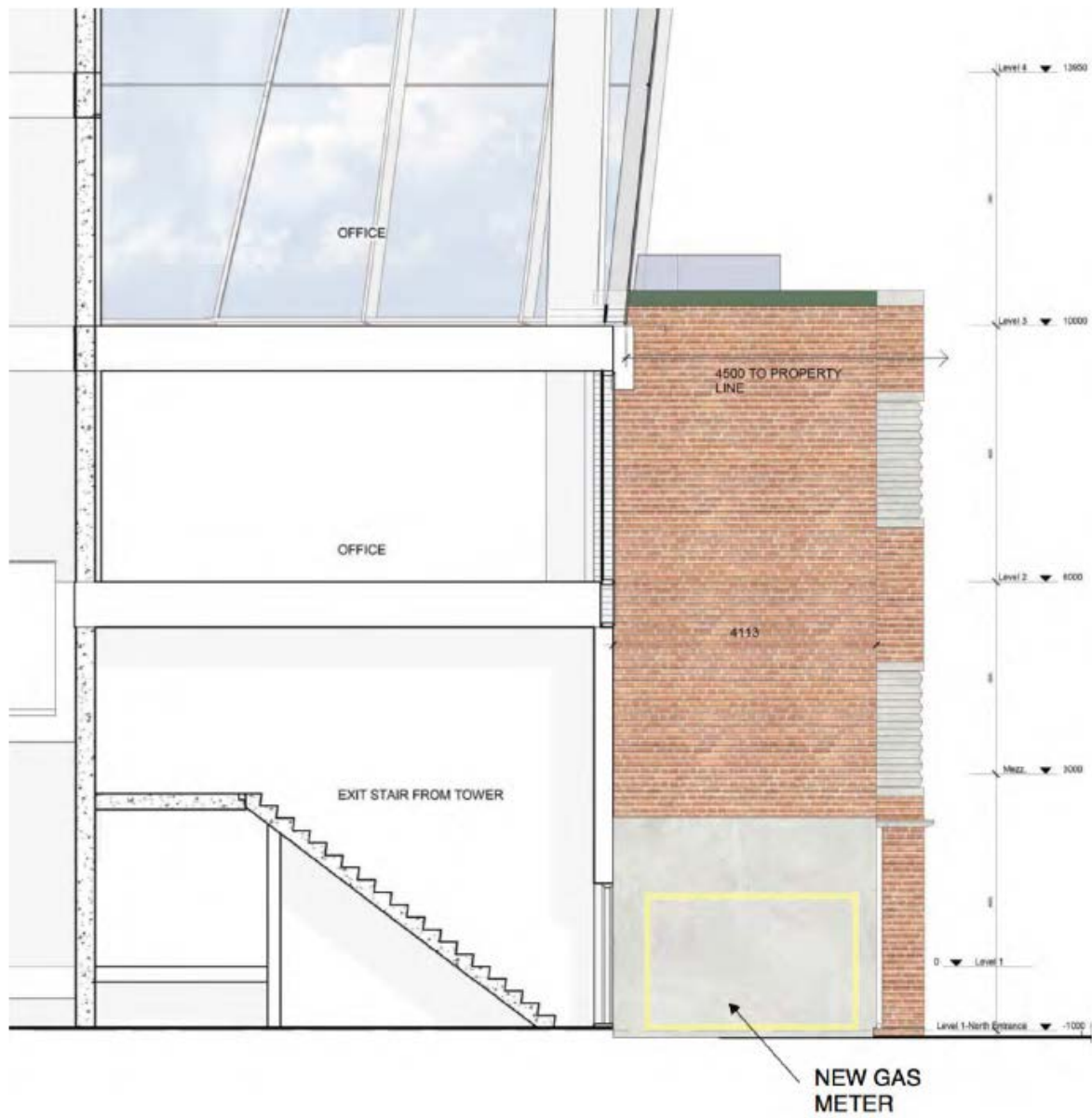
Detail showing the partial reconstruction of the east return wall.
