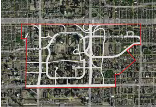
Coarse street network with large blocks & single-use buildings
