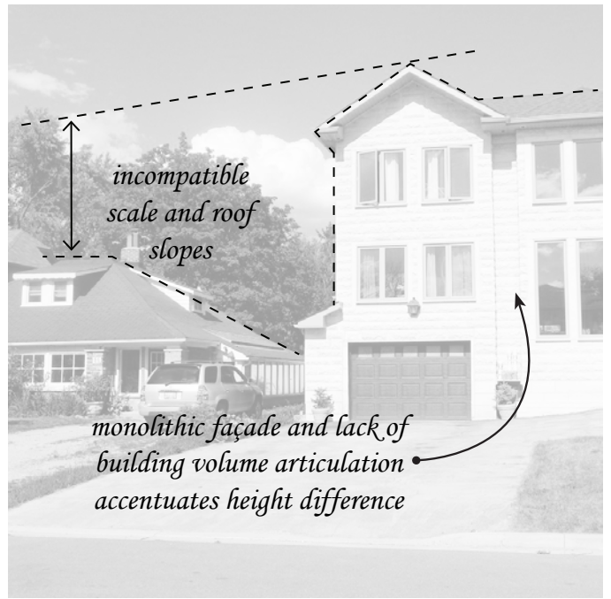
Figure 45 Incompatible building volumes accentuate height difference
