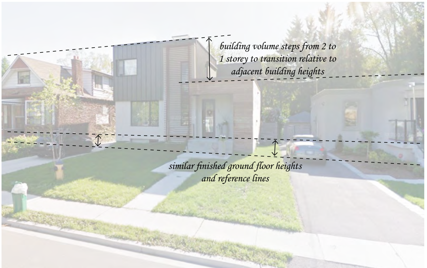
Figure 46 New development transitions height in relation to adjacent buildings
