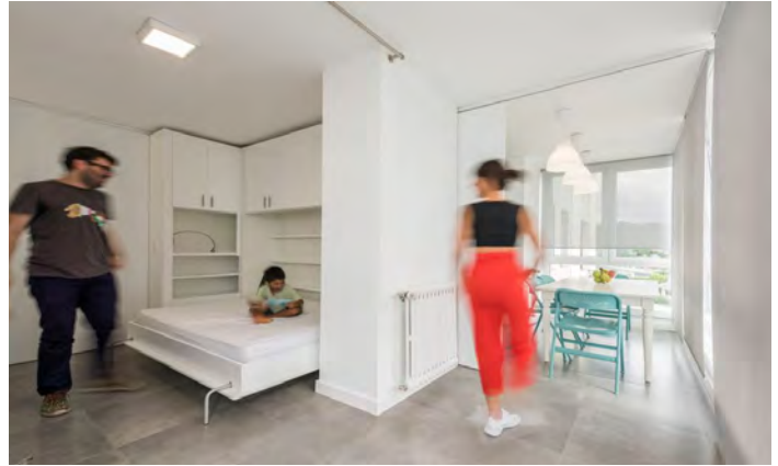
IKEA and PKMN Architects are testing movable walls and fold-away furniture for modifying small spaces. This emerging technology offer an inexpensive solution for adding flexibility to the unit.
