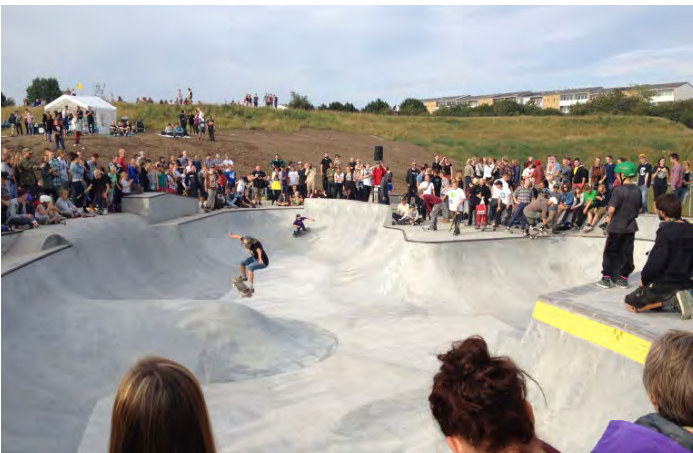
This skateboard park in Roskilde, Denmark functions as a floodwater drainage tool: the basin stores water when it rains and skaters can use the space when it's dry. The basin raises awareness about the need for storm water management.
