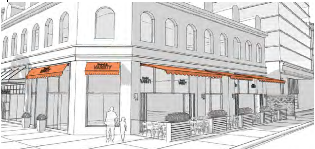
A variety of overhang types incorporated into one retail façade.
