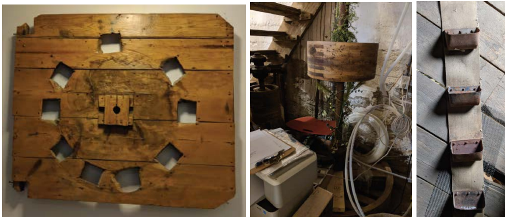
Figure 25. Sorter piece within the distributor (left), a remnant mill wheel (middle), and the scoops and belt for the elevator leg (right) (ERA, 2018)
