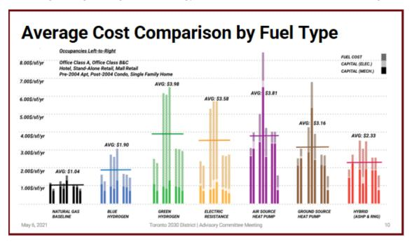
In addition to the costs, we assessed the practicality of building out the distribution system for each energy scenario, and determined that the two most practical were complete electrification based on cold climate heat pumps, and a hybrid system of green gas and standard heat pumps. We also determined that, for both these systems, we already have the distribution systems in place, and it was
