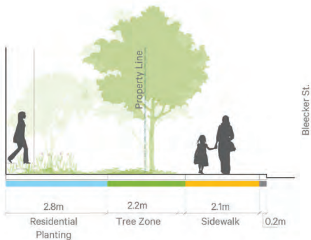
Figure 29: Cross Section E-E Across Bleeker St.
