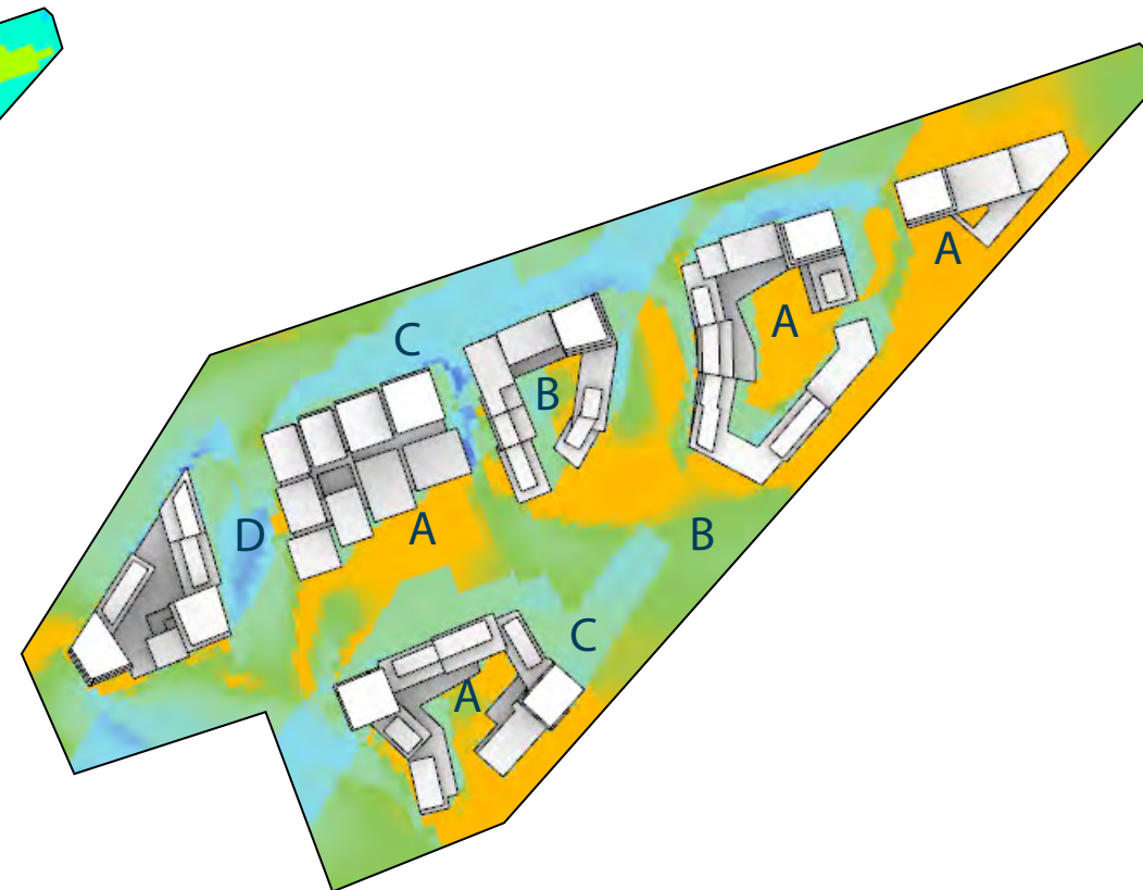
Based on air temperature, solar radiation, wind speed and humidity, this simulation assesses the perceived temperature on an average March day at 2PM
