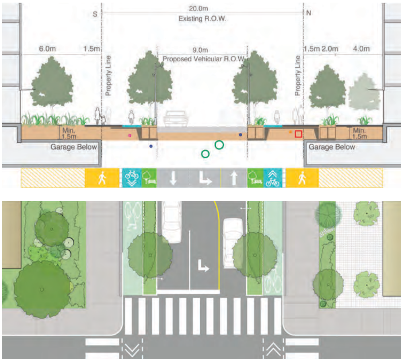
Figure 64 Section and Plan of Broadway Avenue - Recommended Final Condition at intersection with Mount Pleasant Road
