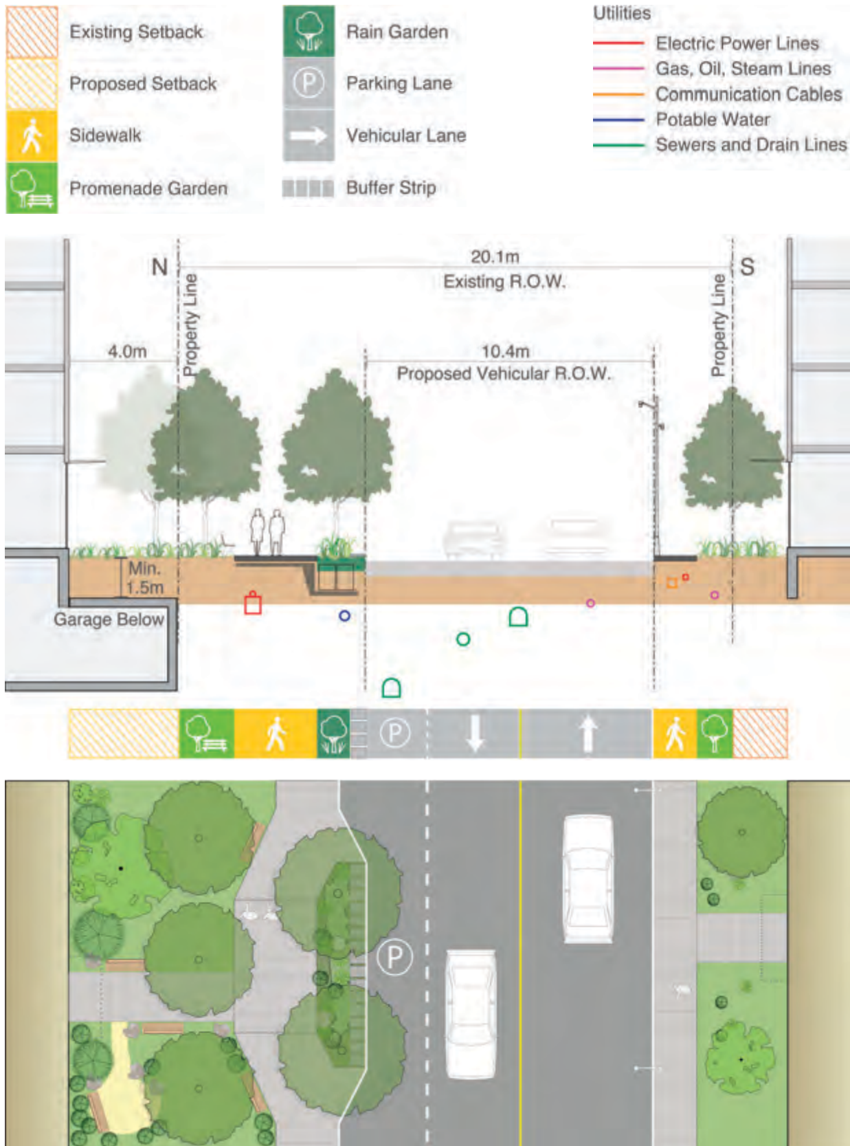
Figure 138 Section and Plan of Merton Street Promenade - Recommended Interim Condition on the north side of the street to be implemented by development
