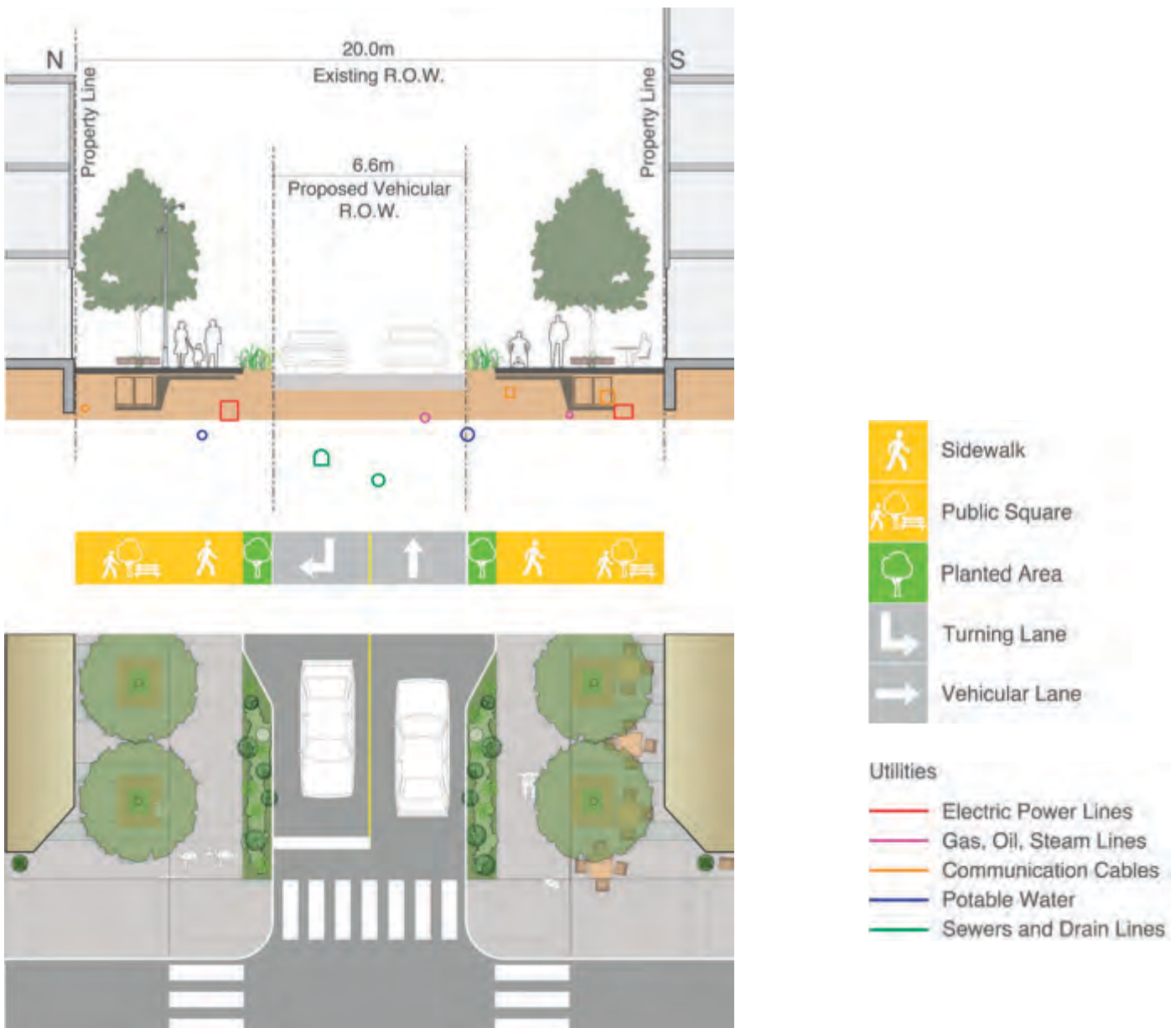
Figure 216 Section and Plan of Erskine Greenway - Recommended Final Condition at major intersections with constrained sites
