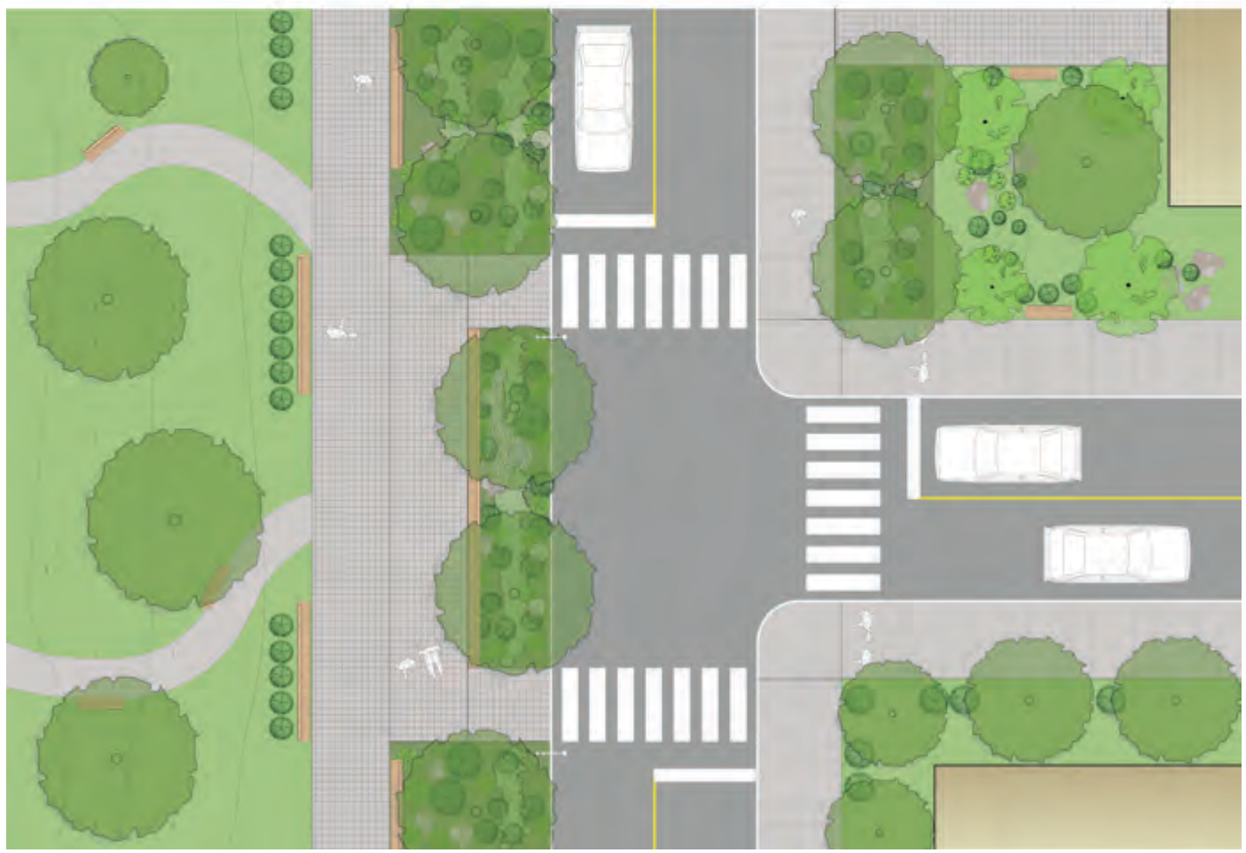
Figure 215 Section and Plan of Erskine Greenway - Recommended Final Condition at bump-out in front of parks
