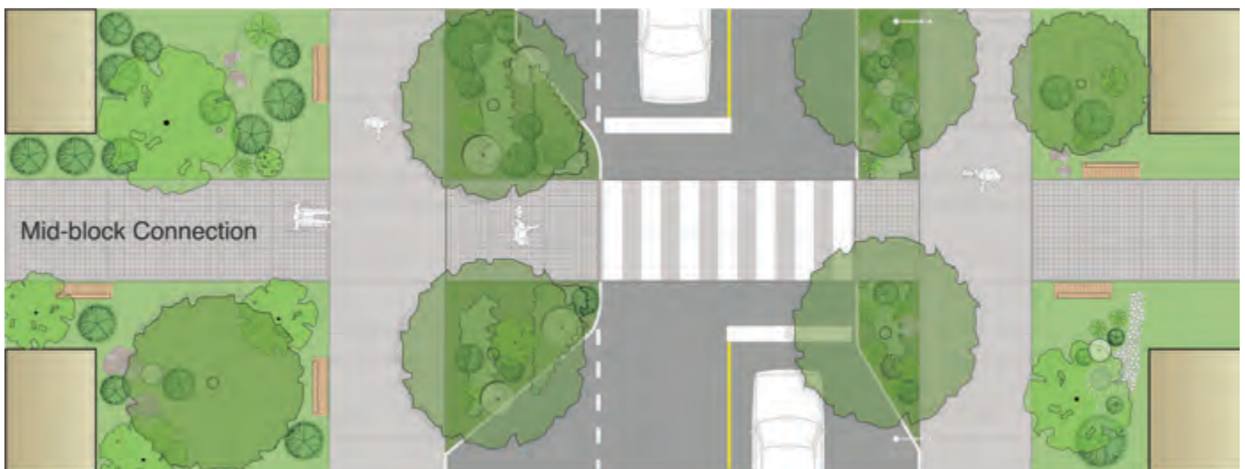
Figure 137 Plan of Merton Street Promenade - Recommended Final Condition of bump-out and raised crossing at mid-block connection
