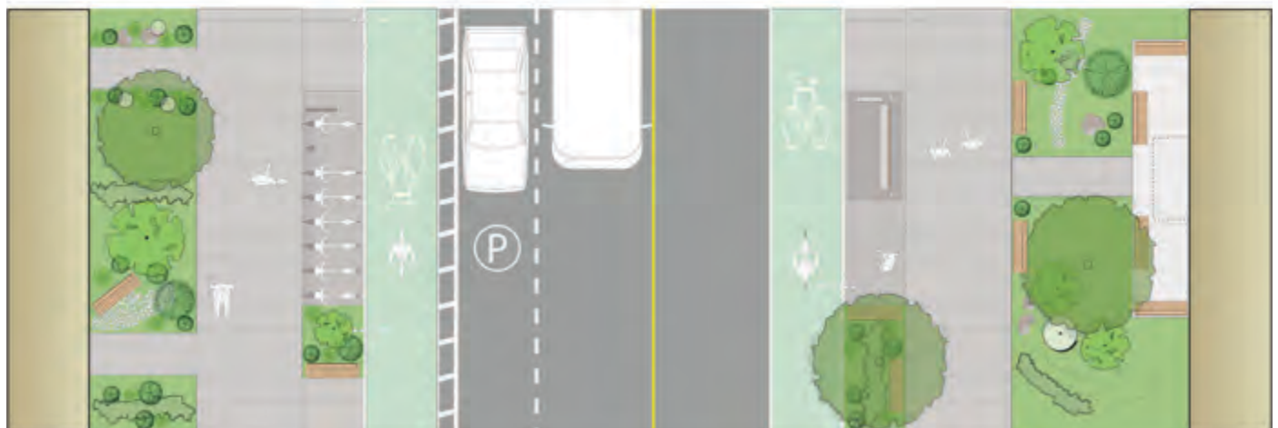
Figure 117 Section and Plan of Green Boulevard and Bike Share Station (North side), and Green Boulevard and TTC Shelter (South side) - Recommended Final Conditions
