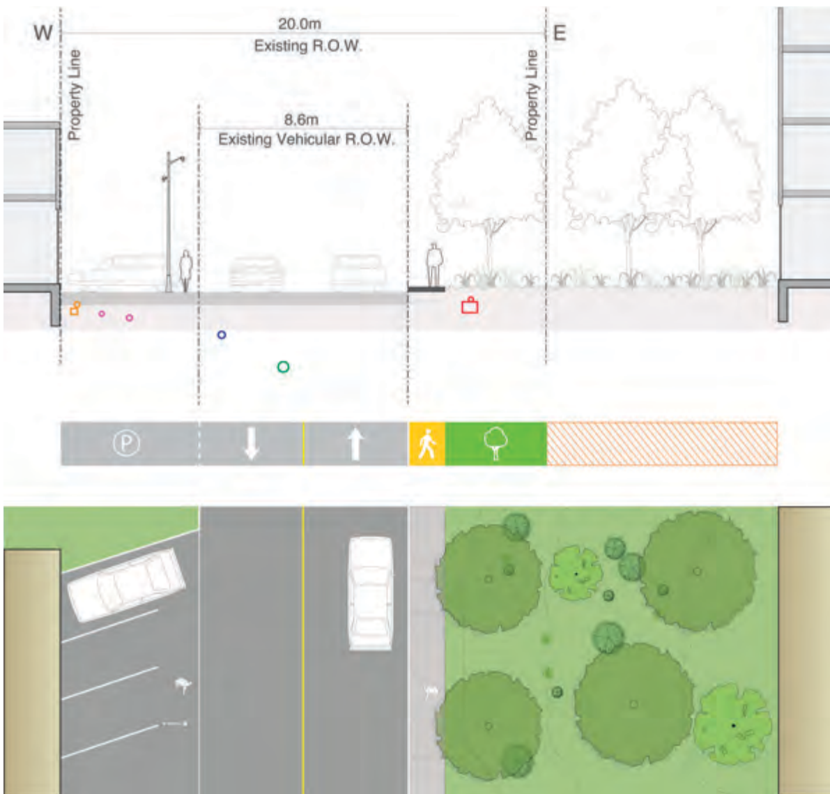
Figure 147 Section and Plan of the Existing Conditions along Pailton Crescent between Balliol and Merton Streets
