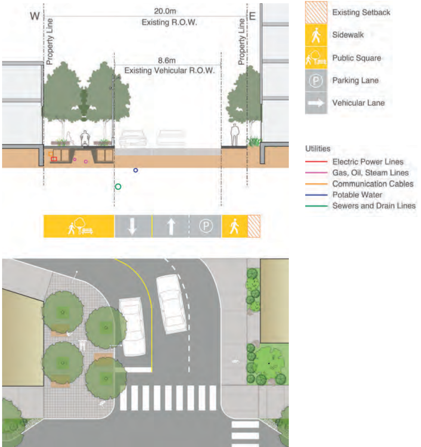
Figure 156 Section and Plan of Pailton Crescent Connector - Recommended Final Condition of public square at intersection with Merton Street
