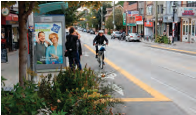
Figure 110 TTC Shelter and raised Bikeway on Roncesvalles Avenue
