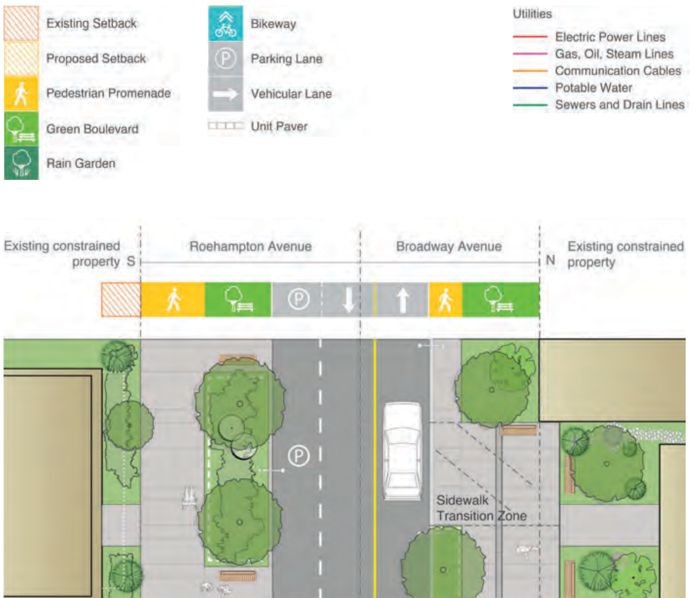
Figure 69 Plan of existing constrained and sidewalk transition - Recommended Final Condition
