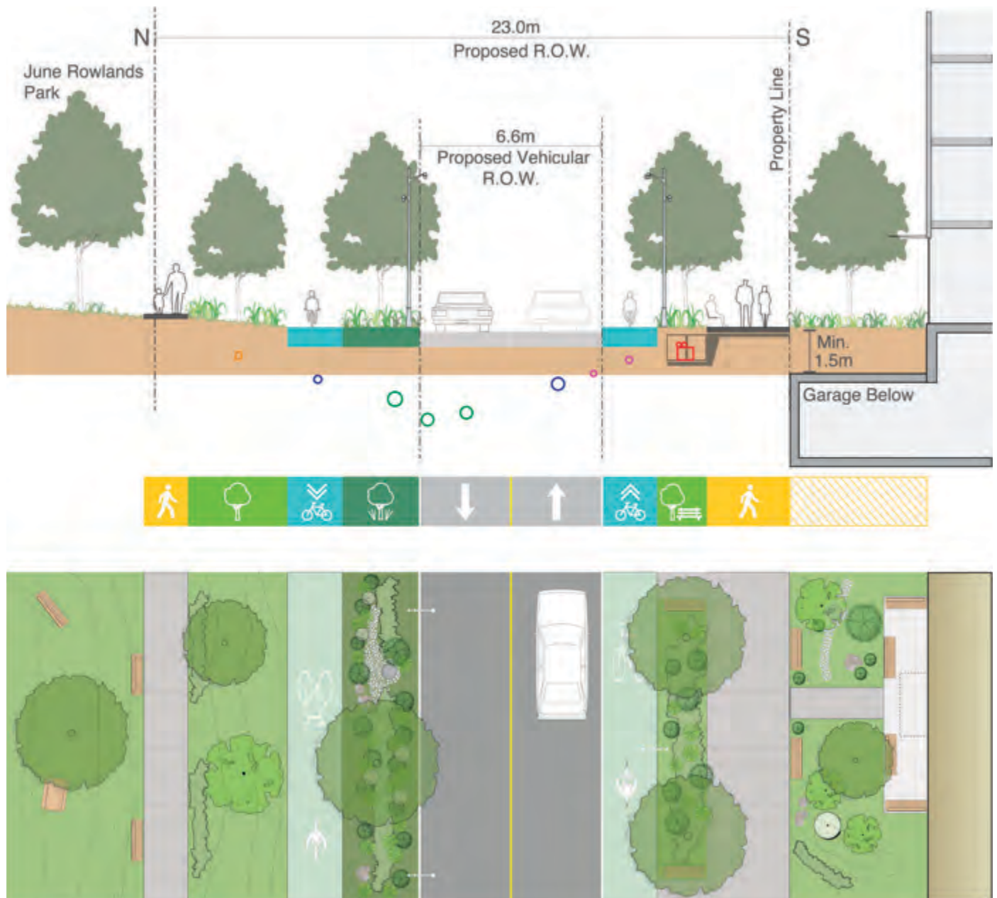
Figure 116 Section and Plan of Davisville Community Street - Recommended Final Condition at bump-out in front of June Rowlands Park
