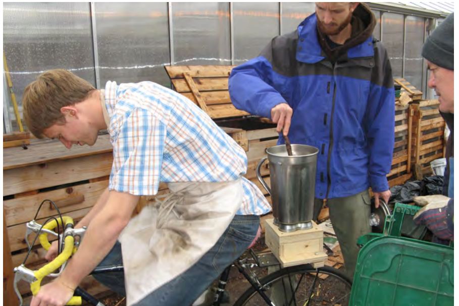
FoodShare built a bicycle-powered wood chipper and shredder which was quickly repurposed into a blender.
