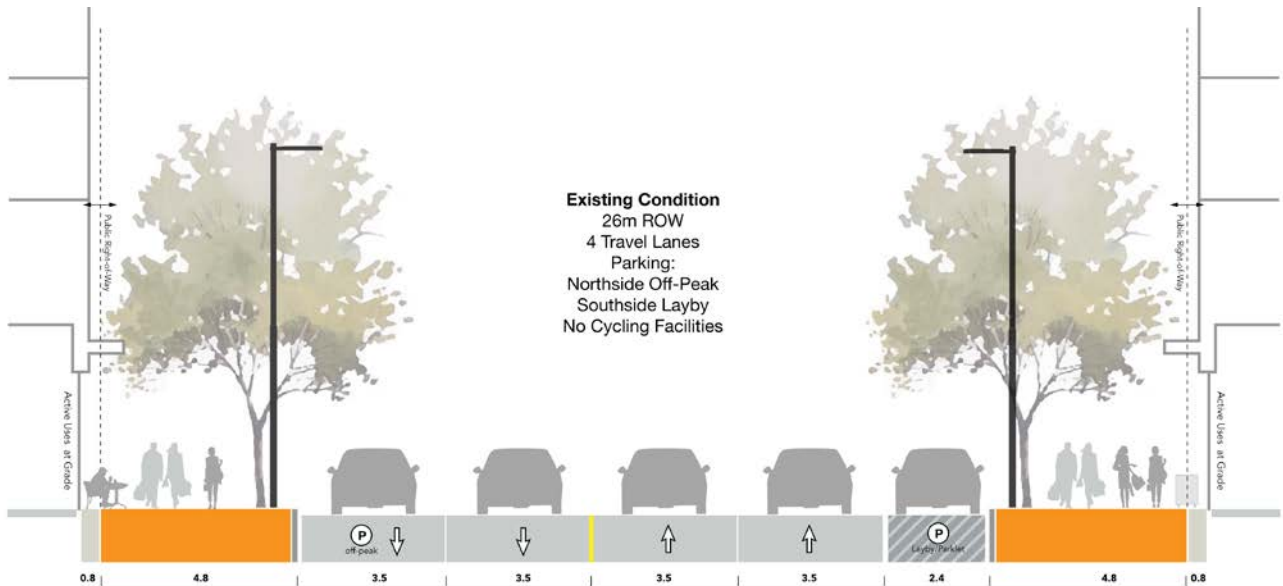
Figure 9: Existing Bloor Street Cross Section (Mid-Block Conditions)
