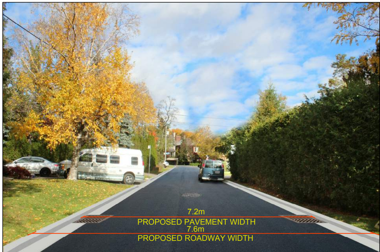
FIGURE LE1 ILLUSTRATION OF EXISTING AND PROPOSED ROAD DIMENSIONS - LEWES CRES
