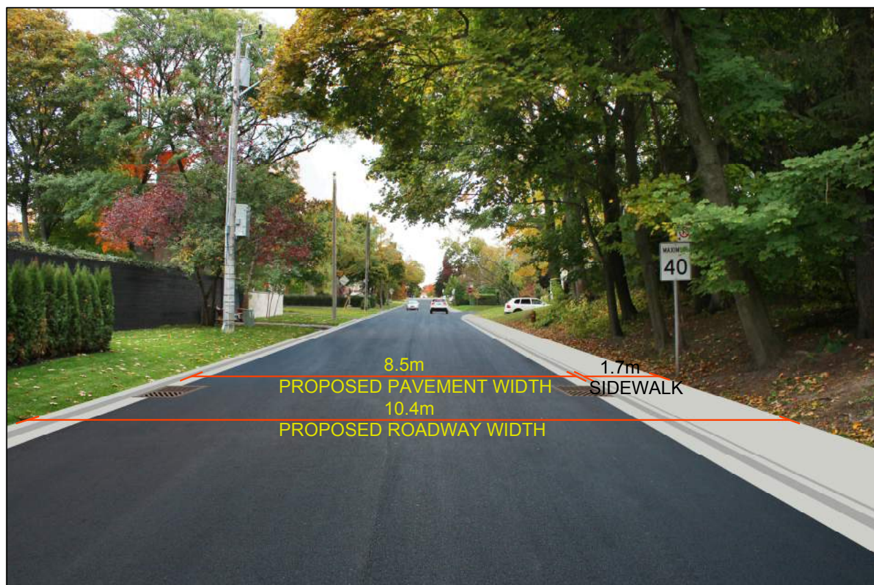
FIGURE ML3-1SW ILLUSTRATION OF EXISTING AND PROPOSED ROAD DIMENSIONS - MILDENHALL ROAD SOUTH OF DAWLISH AVE
