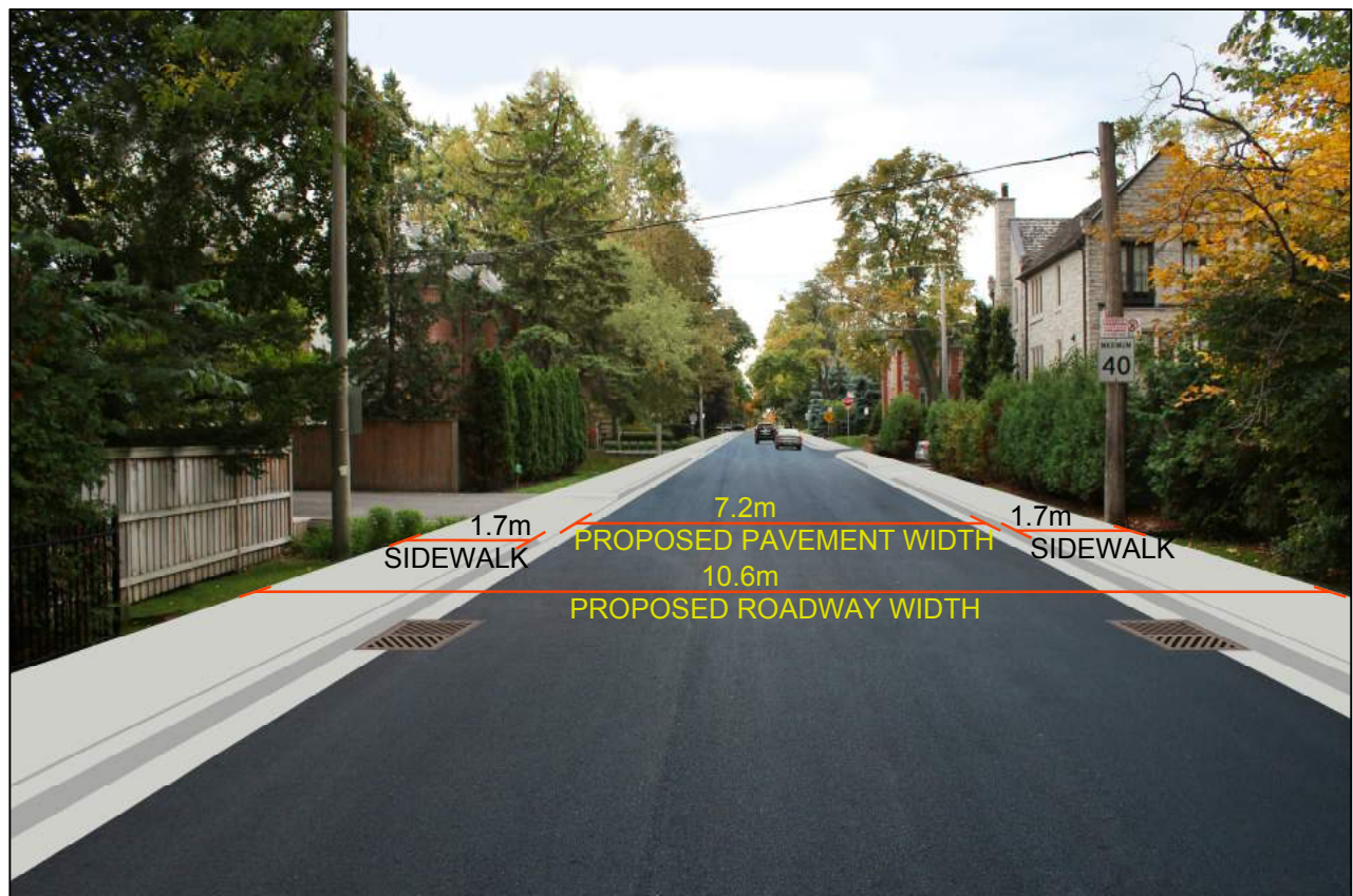
FIGURE ML4-2SW ILLUSTRATION OF EXISTING AND PROPOSED ROAD DIMENSIONS - MILDENHALL ROAD SOUTH OF ROCHESTER AVE
