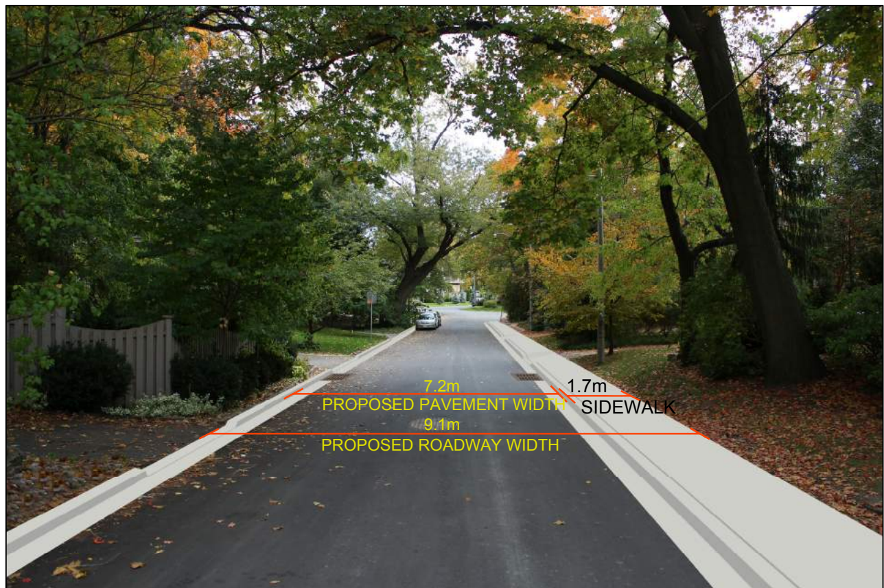
FIGURE PI1 ILLUSTRATION OF EXISTING AND PROPOSED ROAD DIMENSIONS - PINEDALE RD
