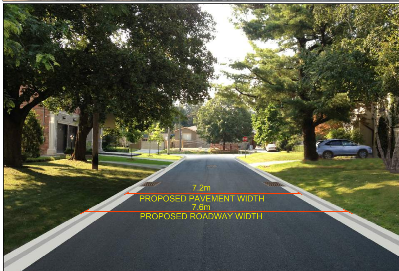
FIGURE PR1 ILLUSTRATION OF EXISTING AND PROPOSED ROAD DIMENSIONS - PROCTOR CRES
