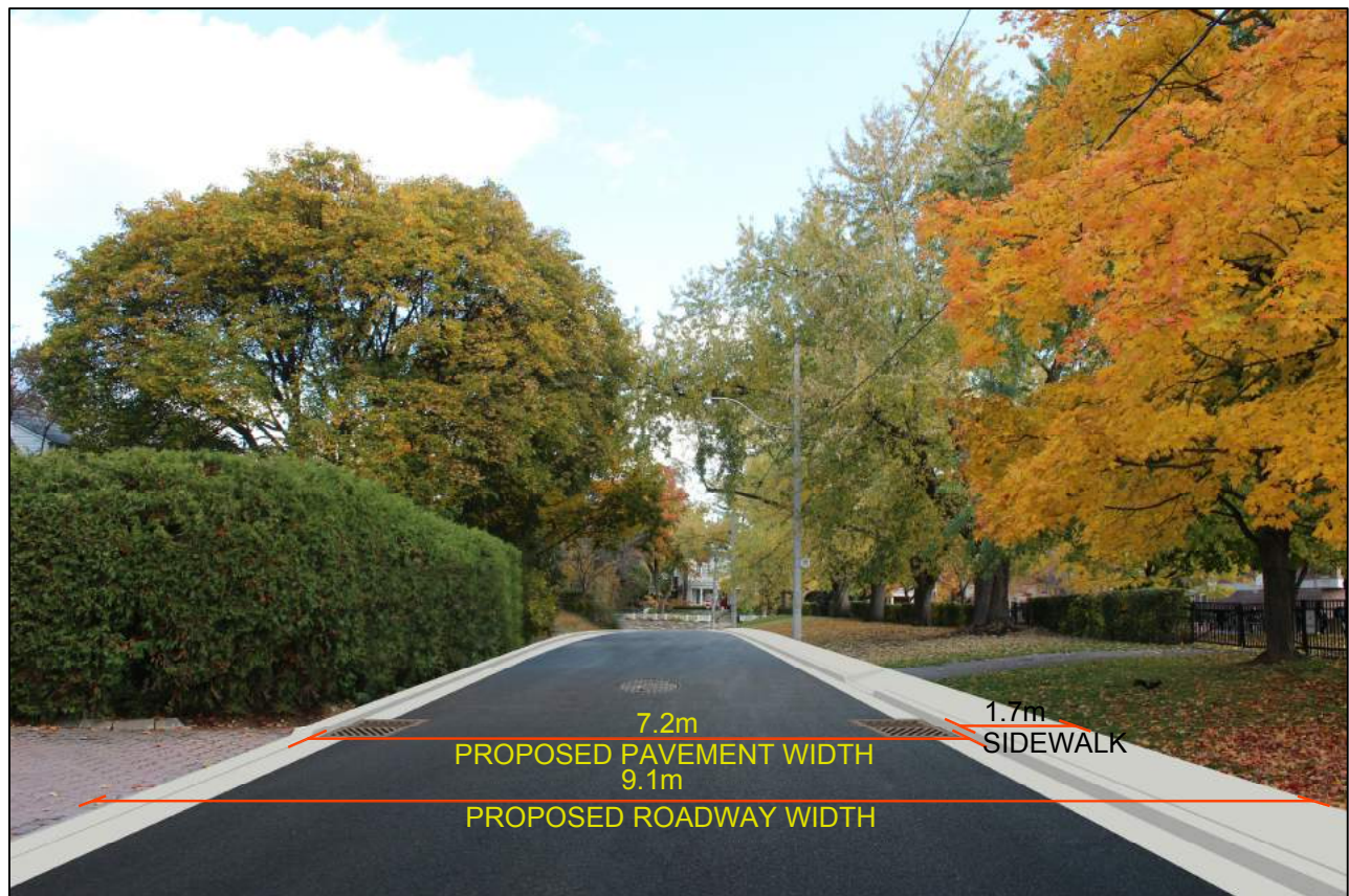
FIGURE GA1 ILLUSTRATION OF EXISTING AND PROPOSED ROAD DIMENSIONS - STRATHGOWAN AVE
