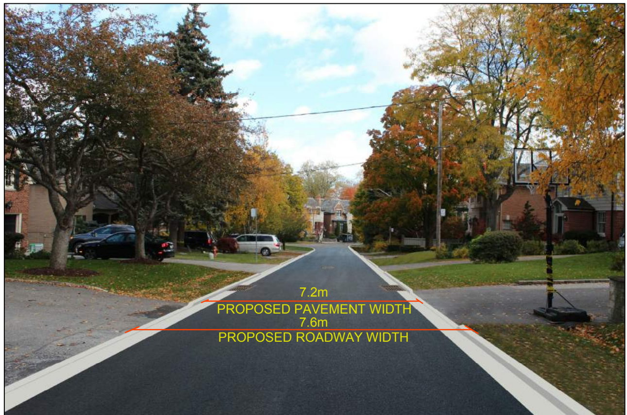
FIGURE BD1 ILLUSTRATION OF EXISTING AND PROPOSED ROAD DIMENSIONS - BLANCHARD RD
