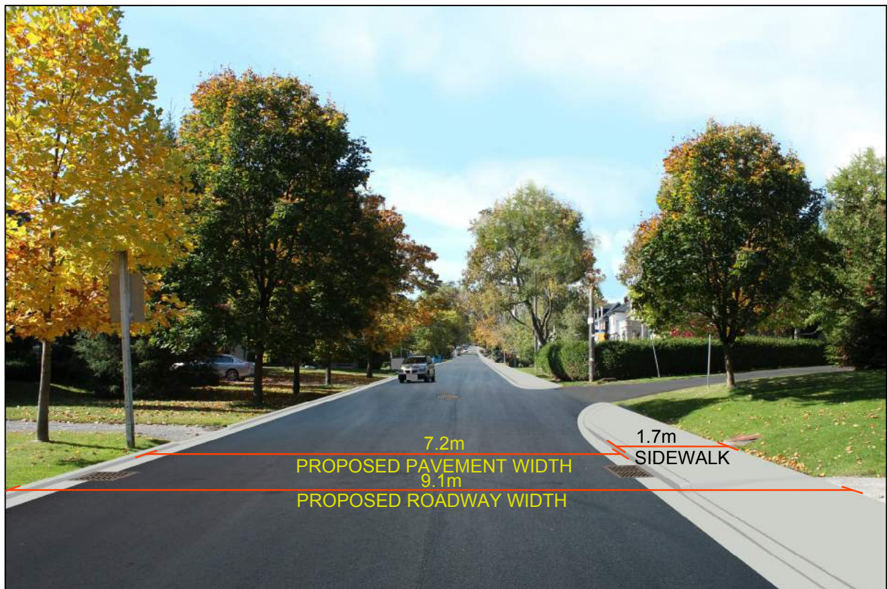
FIGURE SL3 ILLUSTRATION OF EXISTING AND PROPOSED ROAD DIMENSIONS - ST LEONARDS AVE
