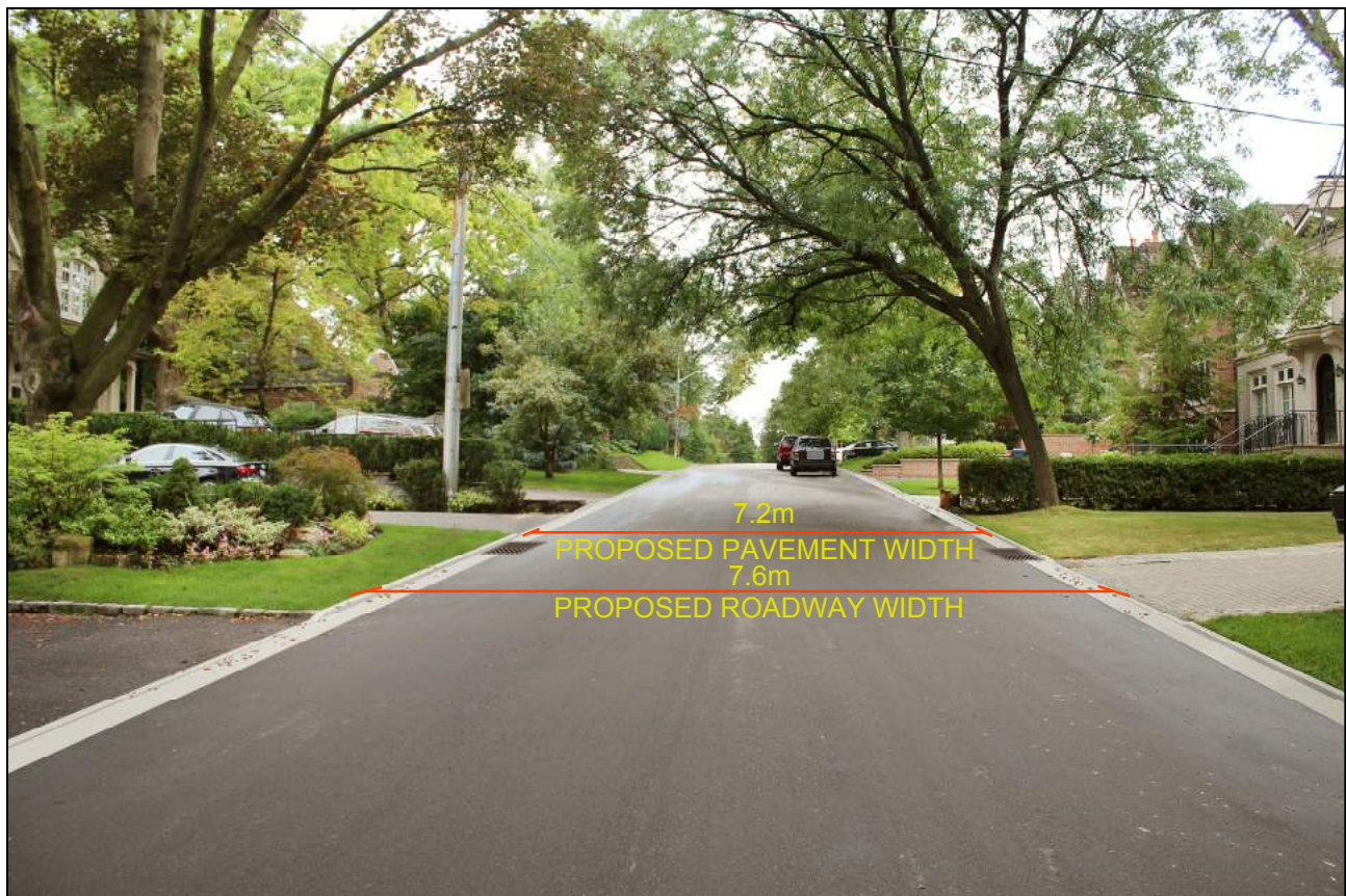
FIGURE CH1 ILLUSTRATION OF EXISTING AND PROPOSED ROAD DIMENSIONS - CHELTENHAM AVE
