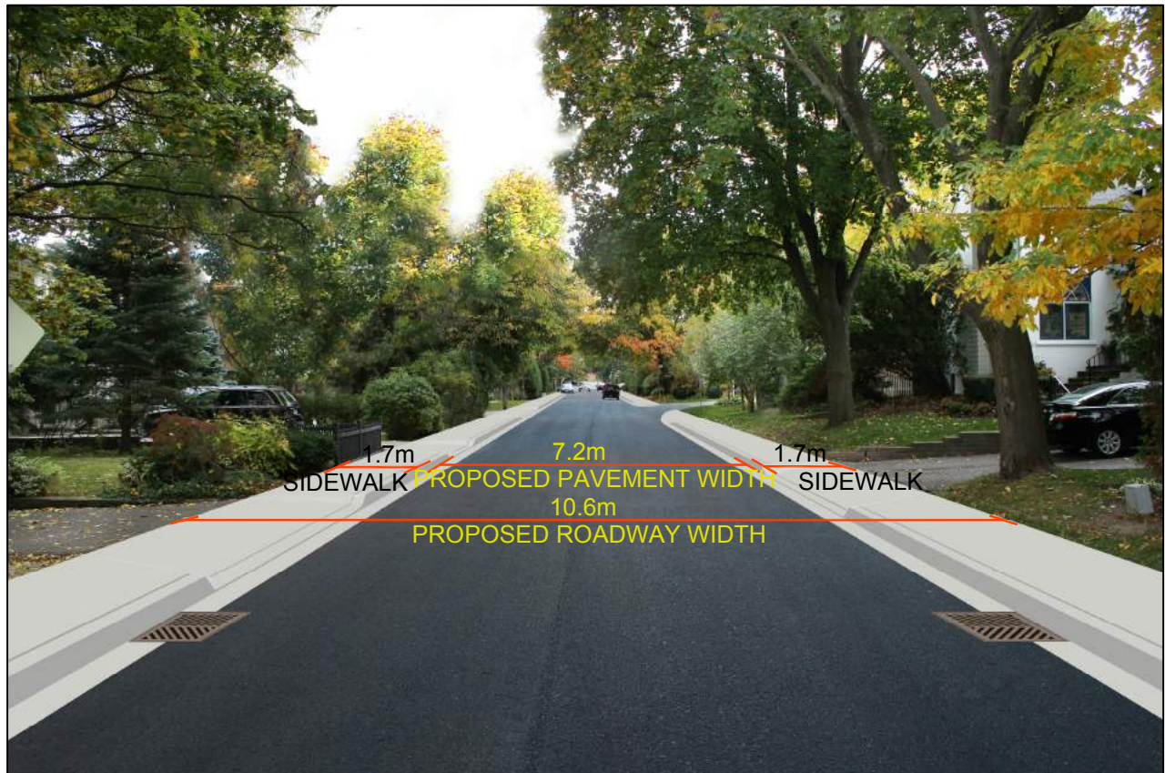
FIGURE ML5-2SW ILLUSTRATION OF EXISTING AND PROPOSED ROAD DIMENSIONS - MILDENHALL ROAD SOUTH OF CHELTENHAM AVE
