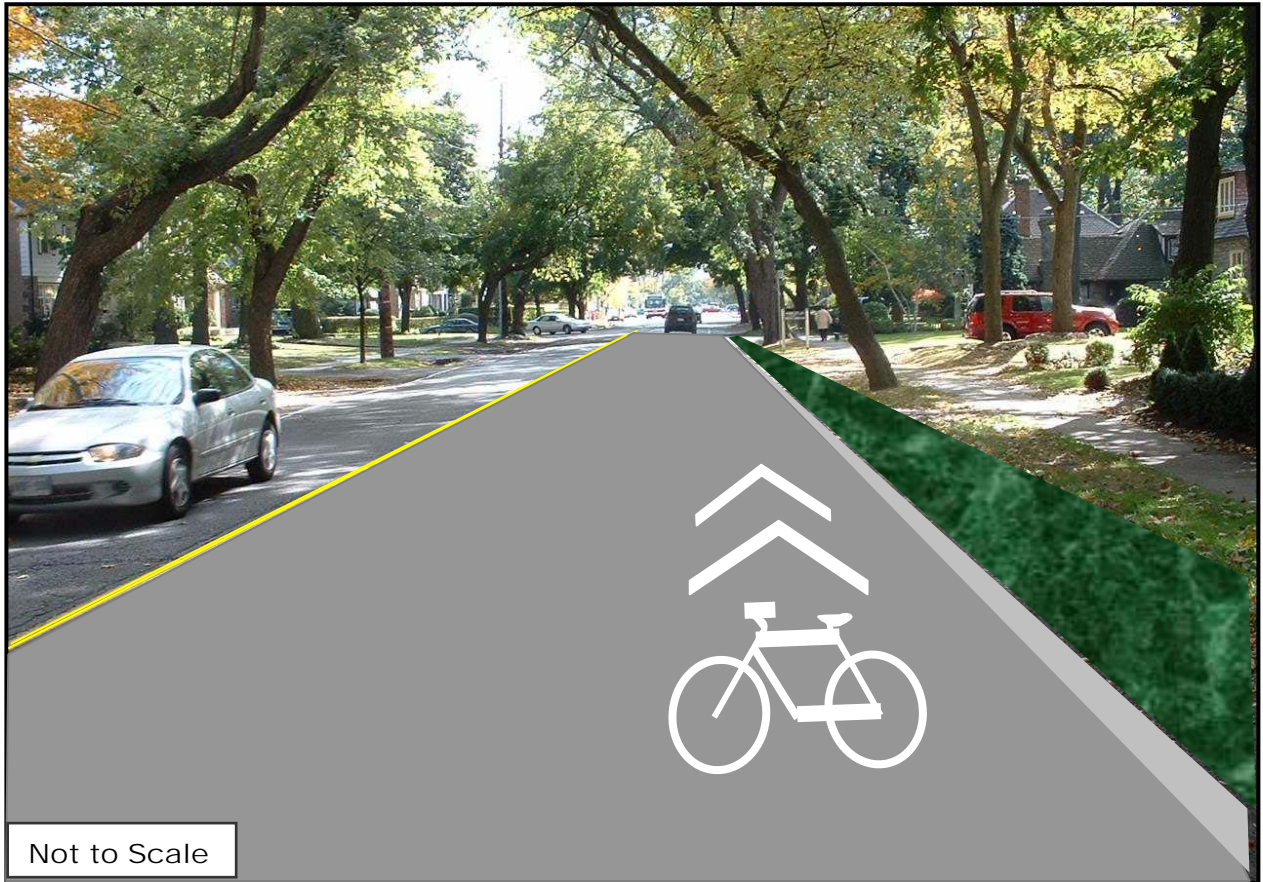
Figure 1: Shared Use Lane Marking
