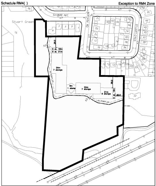
Heights measured from By-law "established grade" of 171.75 A.S.L. to top of main roof slab, excluding height of the mechanical penthouse.
