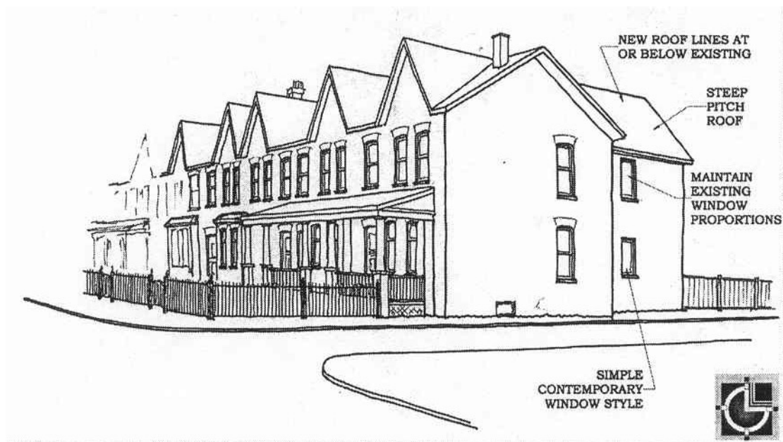
Figure 6. Corner lot, two storey addition to rear elevation of a heritage building.
