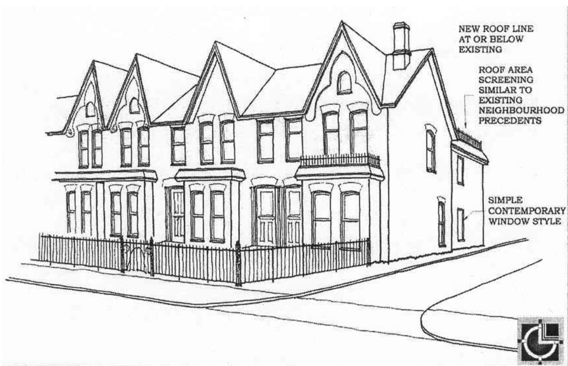
Figure 5. Corner lot, one storey addition to rear elevation of a heritage building.
