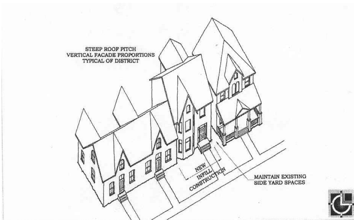
Figure 4. New construction-infill, birdseye view.
