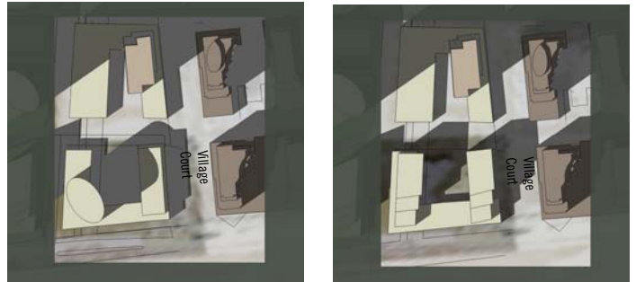
Massing studies for the Village Court shows (left) how moving the density to the other side of the site minimizes shadows (11am)
