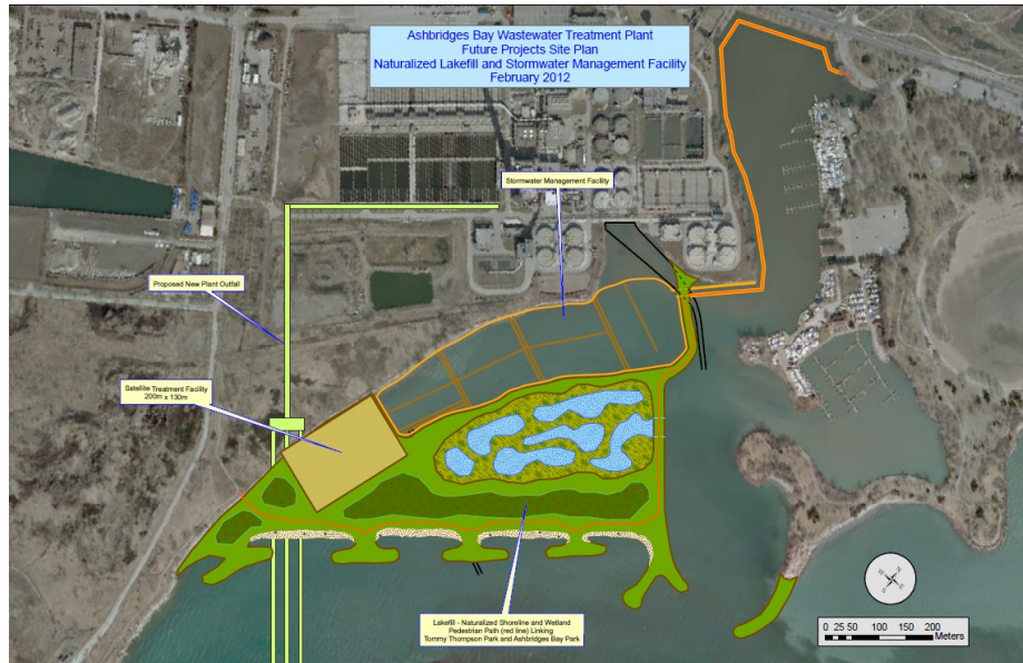
Figure 1 Ashbridges Bay Landform Concept Incorporating Stormwater Management Wetland and Combined Sewer Overflow High Rate Treatment Facility
