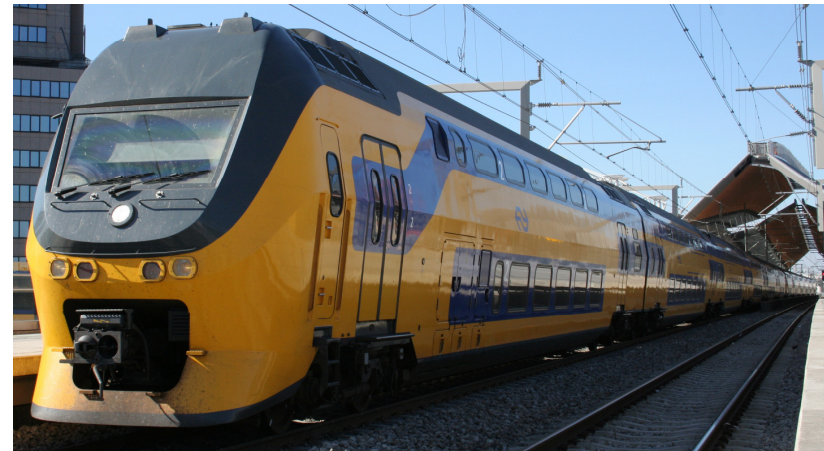
EMU trains criss-cross The Netherlands, with most routes 40-130km long, and a 160km/h (100mph) top speed. A 12-car "VIRM" bi-level EMU train is shown above. Photo credit: Maurits Vink, 2007 Link: en.wikipedia.org/wiki/File:VIRM6.jpg
